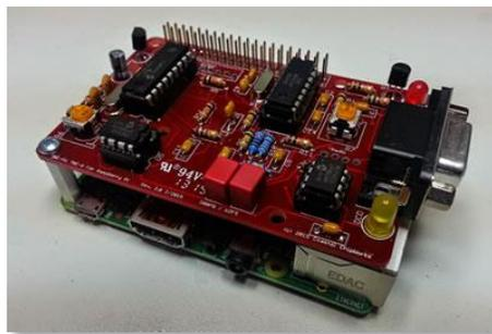
**Figure 2: TNC-Pi 2 mounted on a Raspberry Pi 2.**
