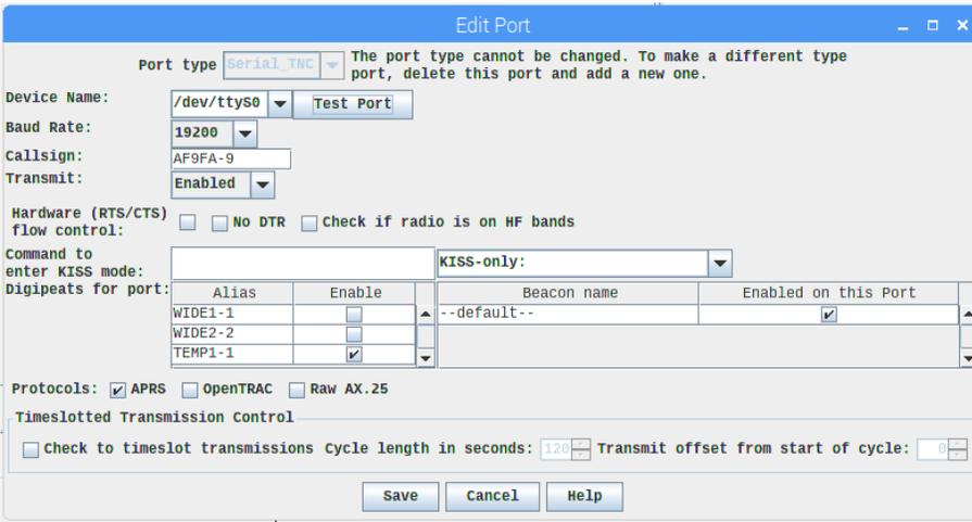
Make sure the rate is set to 19,200. That 's the comm speed used by the TNC-Pi serial connection. The packet speed is 1200 Baud. When you choose the serial port, the laws of the universe state that ALL APRS traffic must stop. your normally noisy radio will go dead silent while testing. I just choose the port and click "Save". There are many more settings under File>Configure. This is documented well on Andrew's website.
