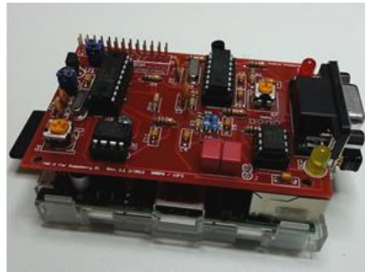
Figure 2: TNC-Pi mounted on a Raspberry Pi
