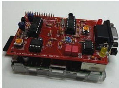
Figure 2: TNC-Pi mounted on a Raspberry Pi
