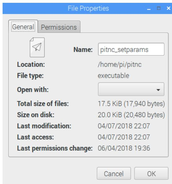
Select the Permissions tab. Change the execute setting from Nobody to Only Owner, and press the OK button. Repeat this procedure with the pitnc\_setparams program.
