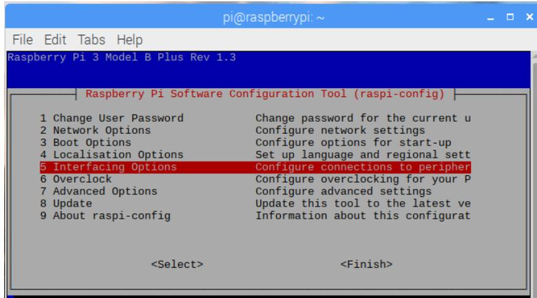
Use the cursor keys to scroll down to Item 5, Interfacing Options. Then, on the next screen scroll down and select P6 Serial.
