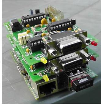
**Figure 1: Two TNC-Pi's stacked on one Raspberry Pi**
